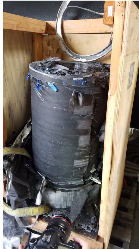
Figure 10. Scale model after implosion (Source: Patrick Loomis)
